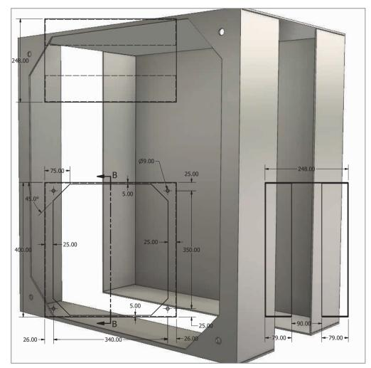
A stainless steel support frame is designed and produced. The frame acts as the structural superstructure to which all outer panels are fixed, leaving the maximum internal volume.
