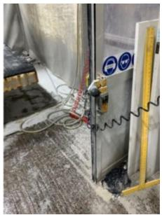
The interlock guard on the sliding doors wasn't working
