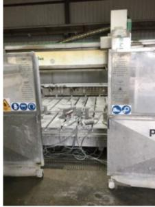
There was no interlock guard on the sliding doors meaning they could be opened while the machine was in operation
