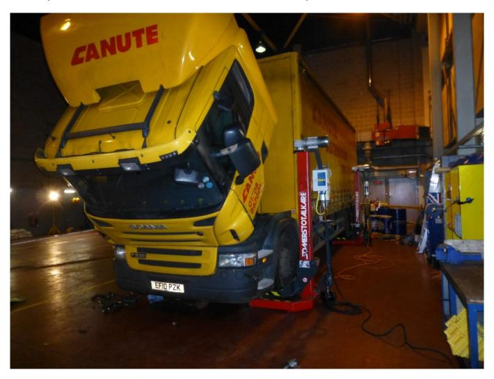
An investigation by the Health and Safety Executive (HSE) found that a cable reel drum jack was used to support the vehicle, which was not an appropriate piece of equipment for the task being undertaken.
