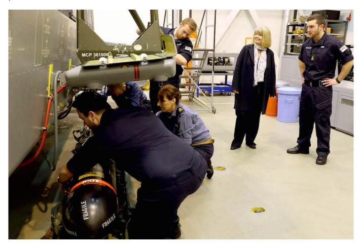
A weapon being loaded onto the Merlin Weapons Systems Trainer. Crown Copyright.
