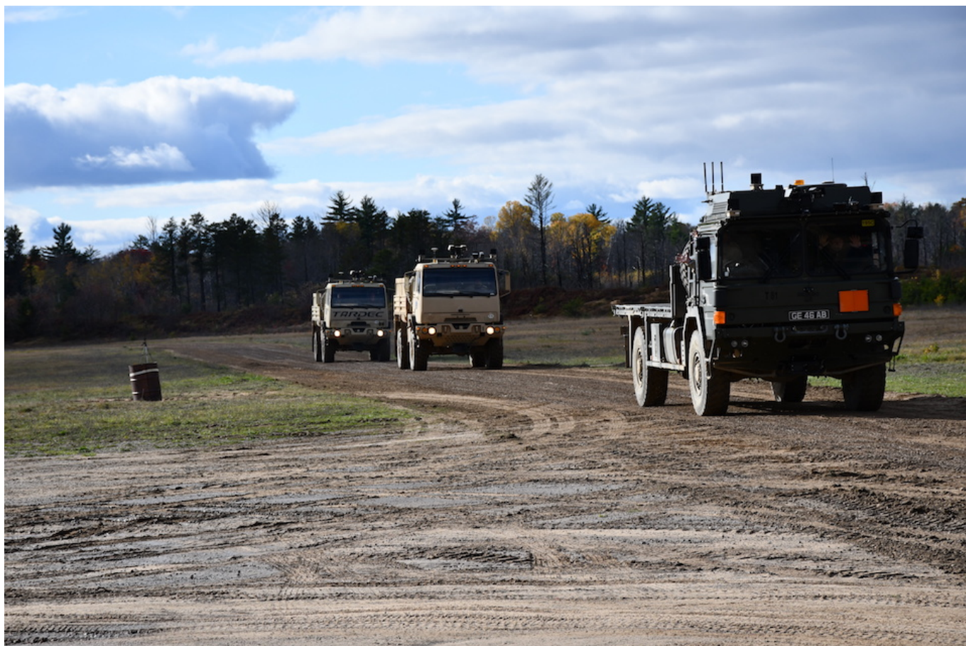
A British Army MAN SV 6-tonne truck leading two US Light Medium Tactical Vehicle trucks in a driverless convoy.
