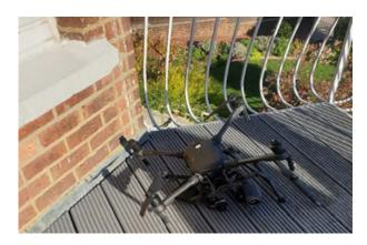
A DJI Matrice M210 Version 1, quadcopter unmanned aircraft (UA) was being flown during a police operation when the wind at 400 ft exceeded the forecast wind, the manufacturer's wind limit and the maximum restricted speed of the UA. The UA drifted beyond visual line of sight and then communication with it was lost. When the battery level was low it entered an auto-land mode but collided with the wall of a house, damaging its propeller blades before coming to rest on a balcony.
