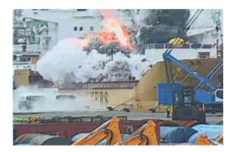
Tank rupture and ignition of released vapour on Stolt Groenland
