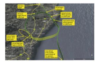
During a go-around at Aberdeen Airport, the aircraft descended from the go-around altitude for around a minute before subsequently climbing. The six crew members and all passengers were unharmed.
