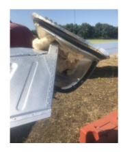
A Mooney M20K aircraft (G-OSUS) had been flying for approximately 15 minutes and was in level flight when the baggage door opened and detached. It struck the right tailplane and remained wrapped round the leading edge near its tip. This caused the pilot control difficulties and increased drag. The pilot declared a MAYDAY and made a successful emergency landing at Membury Airfield.
