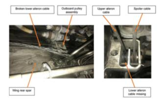
Shortly after takeoff in a strong crosswind, the pilots of a De Havilland Canada Dash 8-402 noticed that both handwheels (control wheels / yokes) were offset to the right in order to maintain wings level flight. The aircraft diverted to Exeter Airport where it made an uneventful landing.
