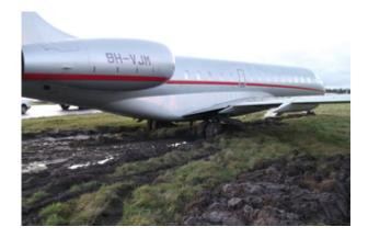
The aircraft, a Bombardier BD-700-1A10 Global 6000 (9H-VJM), suffered a nosewheel steering failure shortly after touchdown. During the subsequent landing roll, directional control was lost due to the inadvertent application of right braking and the aircraft departed the runway surface onto the grass.
