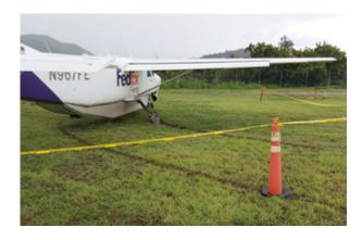
The pilot was operating a cargo flight from San Juan, Puerto Rico to Tortola, British Virgin Islands. He discontinued the first approach due to poor weather. Following the second approach the aircraft made a hard landing that was 795 m beyond the threshold of the 1,206m runway. During the landing roll the aircraft veered off the runway damaging the wheels, landing gear and baggage pod.
