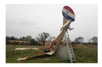
The aircraft, a Replica Royal Aircraft Factory BE2c, was performing a flying display with several other vintage aircraft when it was seen entering a descending right turn. The aircraft did not recover from the descent and struck the ground in a steep nose-down attitude. The pilot suffered serious injuries.
