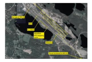
During takeoff, the flight crew inadvertently left the thrust set at the 70% engine run-up setting rather than the 89% required for takeoff. This caused the aircraft to become airborne with only 400 m of runway remaining and climb slowly. At 250ft agl, the flight crew realised they had insufficient thrust and applied the correct power. The flight continued with no further incident and no injuries to the crew.
