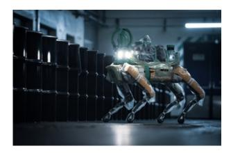
Spot the robot dog made its debut on the Sellafield site in October this year, and has once again been going through its paces by completing its first shift in an active area by collecting valuable information through laser scanning and gamma radiation imaging.
