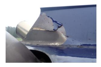
Whilst hovering at 20 ft above ground level, smoke was observed coming from the engine exhaust of an Airbus Helicopters AS355 F1. The pilot was informed and the helicopter landed immediately. After landing a fire was also observed, a fire warning subsequently illuminated, and the pilot activated the fire extinguishing system. The pilot completed the shutdown checks and exited the helicopter. There were no injuries.
