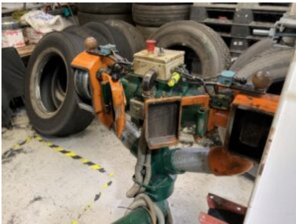
Moveable tyre buffing machine arm with orange rasp covers open
