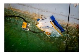
WEDA is a wall cleaning remotely operated vehicle used to clean pond walls on the Sellafield site
