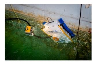
WEDA is a wall cleaning remotely operated vehicle used to clean pond walls on the Sellafield site
