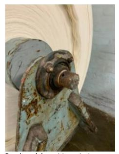
During his attempt to manually slow the rotation of the machine, his sleeve became caught up with an exposed grooved spindle
