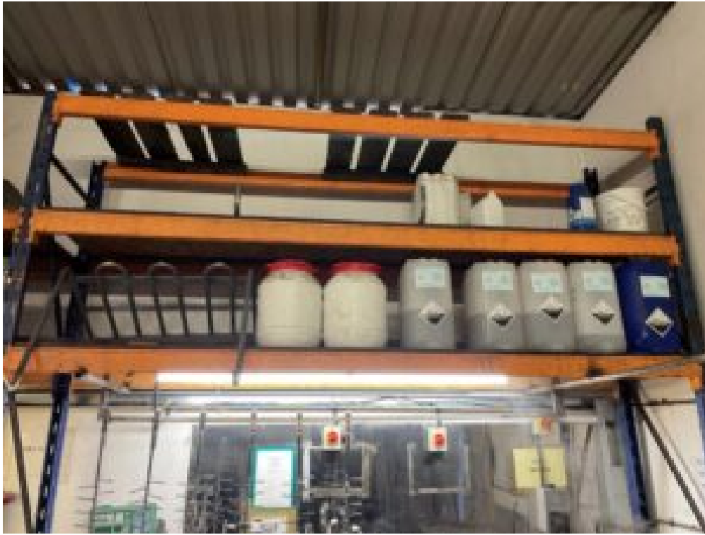
Acids being stored at a high level
