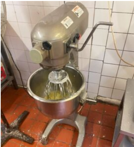
Planetary Mixer missing guard
