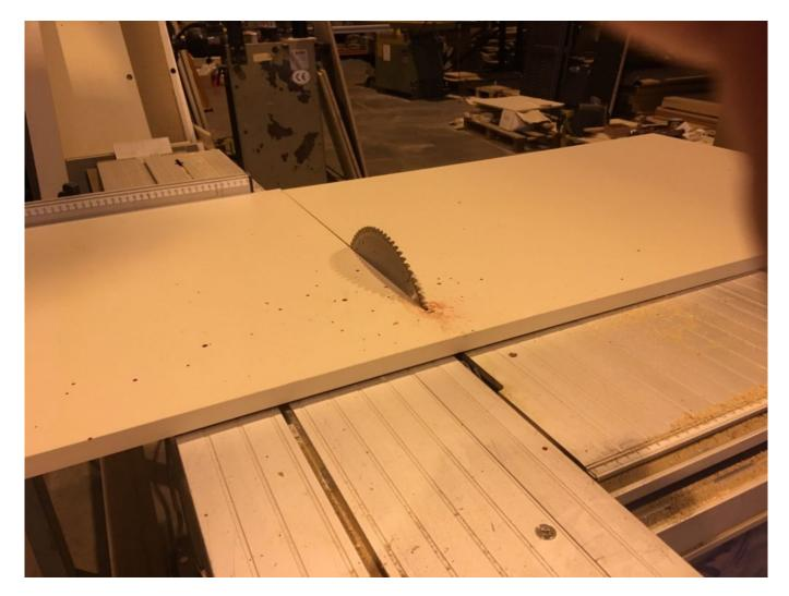
An investigation by the Health and Safety Executive (HSE) found that the worker was pushing the sheets through the saw by hand, without using an appropriate pushstick or jig which would have kept his hand and fingers away from the moving blade. At the time of the incident the crown guard and riving knife were also not fixed to the machine. The investigation also found that there was no Employer's Liability (Compulsory Insurance) policy in place.
