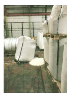
The Health and Safety Executive (HSE) investigation found that the FIBCs were stacked in an unsafe manner at a height of approximately 2.2 metres. The employee reversed the forklift truck and it caught one of the lower FIBCs causing it to tear and spill its contents. The employee attempted to repair the tear but the top FIBC, weighing about 1 tonne, fell and struck the employee.
