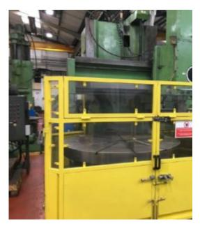
An investigation by the Health and Safety Executive (HSE) into the incident found that the interlocks on the perimeter fencing access doors were not working, and there were no safety checks in place to ensure that the
