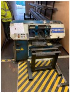
The horizontal band saw the apprentice had been using
