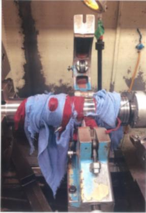
An investigation by the Health and Safety Executive (HSE) found that machinery had interlock devices fitted but they had been by-passed/defeated so it was possible to move guards/doors that should have been interlocked out of the way during set up, to allow access to the rotating chuck and workpiece.
