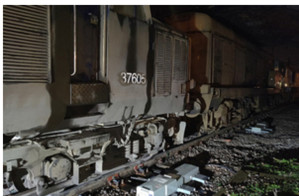
The derailed locomotive
