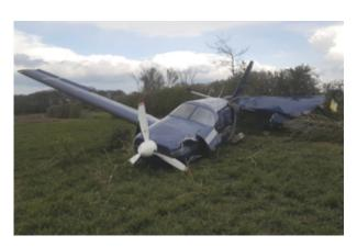
During an experimental flight near Cranfield Airport of a modified Piper PA-46-350P (G-HYZA), an electrically powered aircraft with electrical power from hydrogen fuel cells, suffered a loss of power to the electrical motors. This meant a forced landing was carried out, which severely damaged the aircraft, the crew were unharmed.
