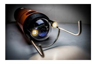
Robots are already in use at Sellafield. For example the Avexis (pictured) offers the ability to 'see' inside a waste silo via cameras attached to its body.
