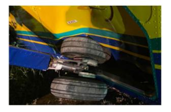
On landing, the pilot was unable to maintain directional control and reported the left brake was 'spongy'. The aircraft veered off the right side of the runway and impacted the bank of an adjacent drainage ditch. One passenger suffered minor injuries as a result.
