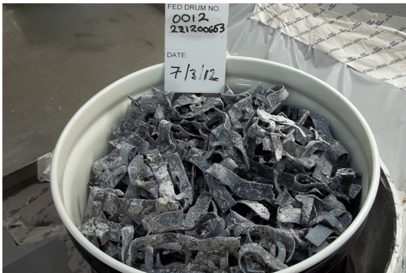
Fuel Element Debris (FED)
