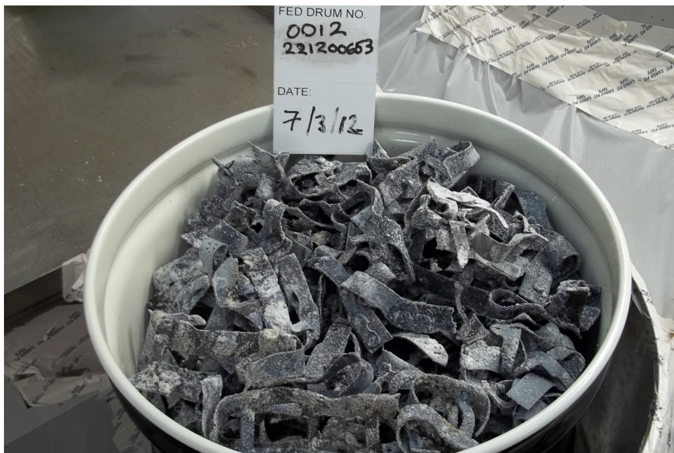
Fuel Element Debris (FED)
