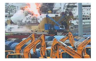
Today we have published our investigation report on the rupture of a cargo tank containing styrene monomer on board the Cayman Islands registered chemical tanker Stolt Groenland on 28 September 2019. The large quantity of vapour released as a result of the catastrophic rupture subsequently ignited, resulting in a fireball. Two crew were injured and fire fighting efforts lasted over 6 hours, with 15 emergency responders also sustaining injuries during the emergency response.
