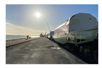
High level waste flasks loaded for transfer to storage site in Germany
