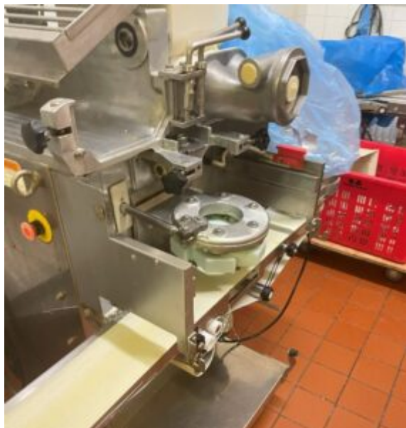
Mochi making machine with missing front guard
