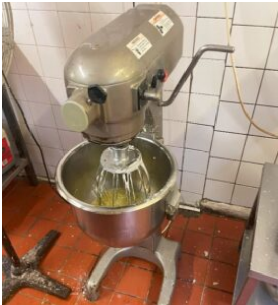
Planetary Mixer missing guard
