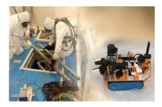
Dounreay Site Restoration Ltd (DSRL) and the Robotics and Artificial Intelligence in Nuclear (RAIN) Hub are working together to develop a robot capable of accessing areas that are inaccessible or unsafe for humans to work in. The RAIN Hub is a consortium of universities led by the University of Manchester.
