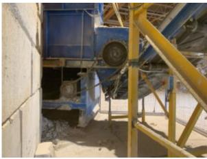
The man's arm became entangled in the trapping point between a conveyor belt and the rotating drum powering the movement of the belt
