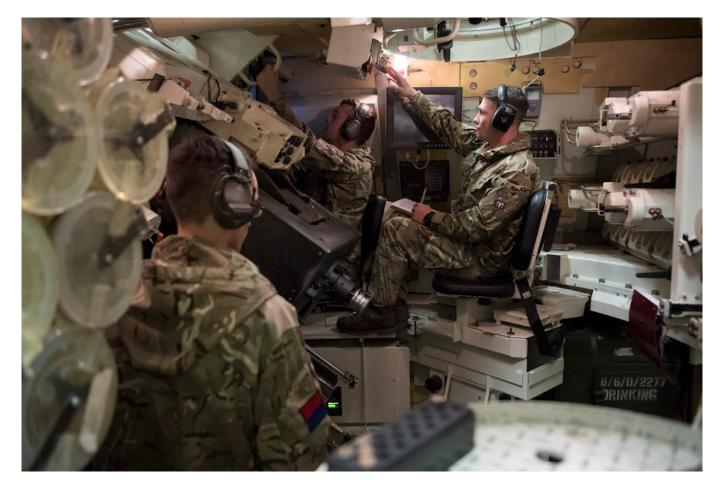
Based on a real AS90 turret, the trainer uses an electro-mechanical system to fully replicate a complete firing cycle. This includes the weight and size of the artillery rounds and the noise and turret movement on firing.
