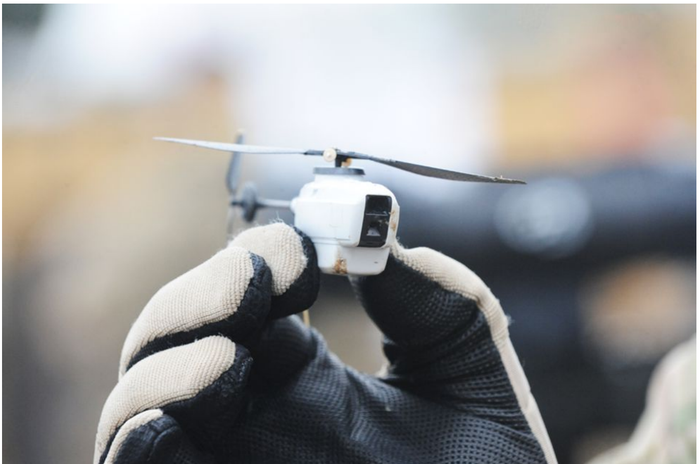
A Black Hornet nano helicopter unmanned aerial vehicle (UAV). Crown Copyright. Photo: via MOD.
