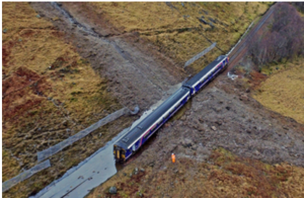
Aerial image of the landslip and derailed train
