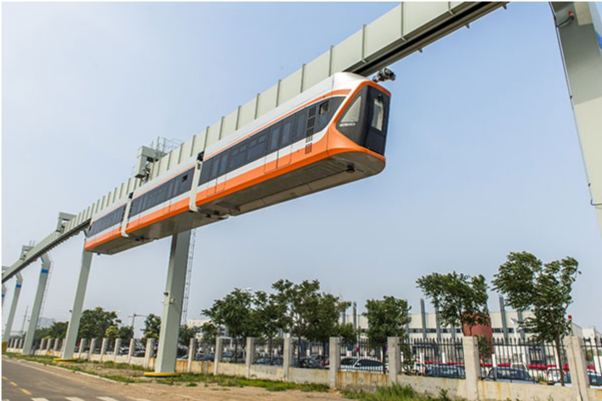
A prototype of a mounted monorail train is tested at CRRQ Qingdao Sifang.[Provided to China Daily]
