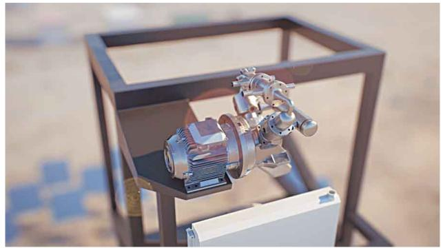
The Stirling engine efficiently converts thermal energy into mechanical movement to generate electricity. (Supplied)
