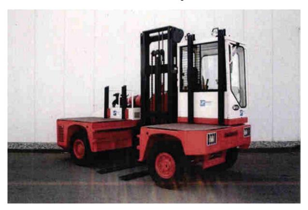
An investigation by the Health and Safety Executive (HSE) identified that the work method used to lift and move the pipes was unsafe. There was no method to secure the pipe on the forks when lifted, which meant when the pipe began to roll along the forks the operator had no control over it. The pipe subsequently fell off the end of the forks, ultimately leading to Mr Longair's fatal injury.
