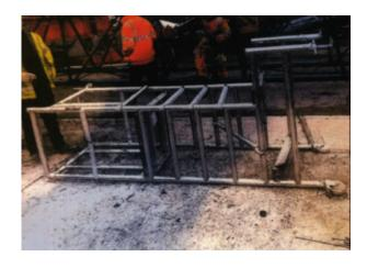
An investigation by the Health and Safety Executive (HSE) found that the company had failed to follow its internal procedures, and did not carry out a risk assessment nor determine a safe system of work. The podium steps had been modified with the addition of incorrect feet, contrary to the manufacturers' instructions. Stabiliser bars had also not been fitted and workers had not been trained in their correct use.
