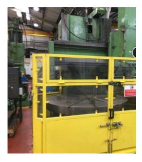
An investigation by the Health and Safety Executive (HSE) into the incident found that the interlocks on the perimeter fencing access doors were not working, and there were no safety checks in place to ensure that the interlocks were in working order.
