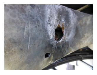
An investigation by the Health and Safety Executive (HSE) found that Unique Envelope Façade Solution Limited's risk assessments and method statements did not consider the risk of drilling into cable trays containing live cables, isolating the electrics to complete work, or other methods of fixing which did not involve drilling.
