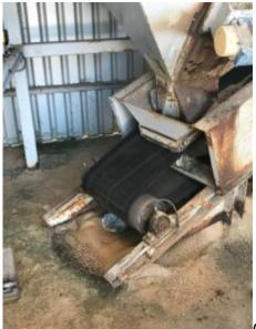
Chelmsford Magistrates' Court heard how, on 18 February 2019, an employee was removing sand from the inside of a conveyor belt in an attempt to fix the machine at Slough Lane, Colchester. The employee's left glove became caught in the in-running nip of the conveyor tail drum, pulling his hand and arm into the machine. The emergency stop button in the building did not work, so a colleague had to run to another building to alert the operator at the control panel to turn the machine off.
