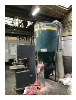
An investigation by the Health and Safety Executive (HSE) found that the blender had not been sufficiently guarded to prevent access to dangerous parts of machinery. There was a large gap of approximately  $4 \times 5$  inches towards the top of the hopper guard. The injured employee had only been operating the machine for one week prior to the incident.
