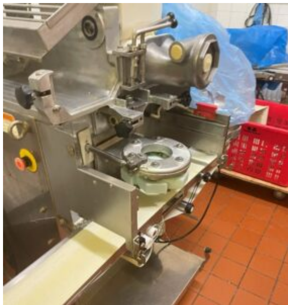
Mochi making machine with missing front guard
