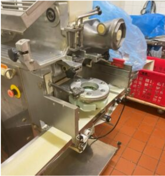
Mochi making machine with missing front guard
