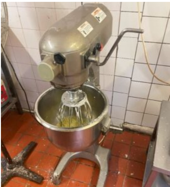
Planetary Mixer missing guard
