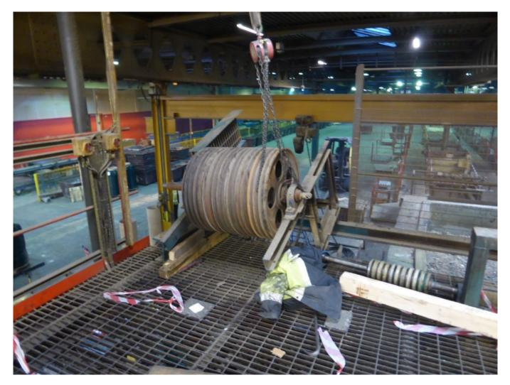
He unbolted the two parts, with a colleague using a fork lift truck to hold the weight of the quench unit. As they separated, the metal carriage which held the roller tilted forward. The roller landed on his lower back. He suffered fractures of his pelvis and lumbar region of his spine.
