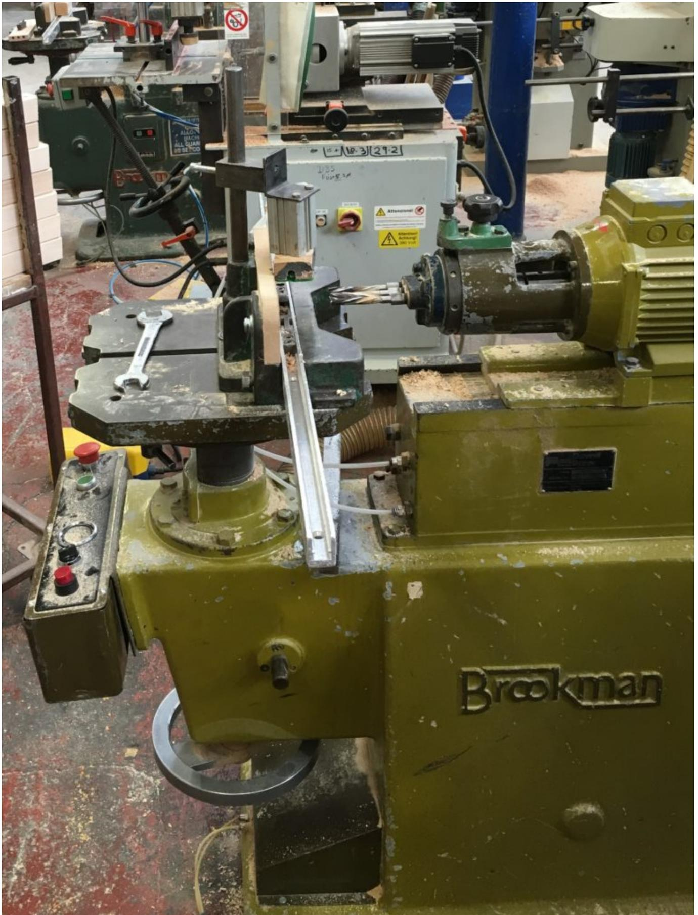
The Health and Safety Executive (HSE) investigation found that it was possible for employees to reach the dangerous parts of the horizontal drilling machine when it was in operation as A and L Furnishings Ltd had failed to provide a suitable guard for the machine.
